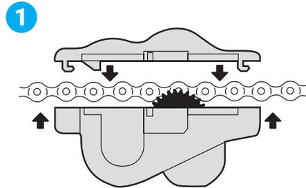
Open the case and lay the chain as it is shown into the guide. Make sure that the fastening rail of the handle points in your direction. Close the cover of the case and check the correct closure.
