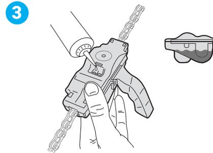
The casing can now be filled with chain cleaning fluid through the openings on the top. To avoid unnecessary leakage, fill up to the maximum of the displayed mark on the illustration.
