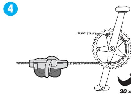
Hold the filled case by the handle while moving the pedals 30 times around their own axis with a steady even speed, pulling the chain through the chain cleaner.
