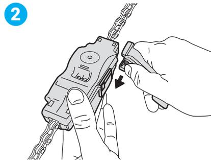
Slide the handle as shown on the prefabricated rail until it clicks into place.
